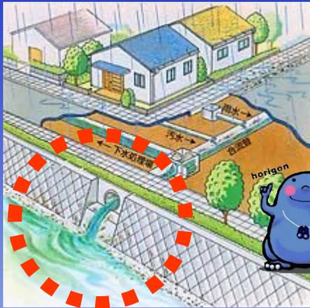
Less than certain amount of rainwater is treated with wastewater in water treatment center, but more amount is directly discharged into the river.
