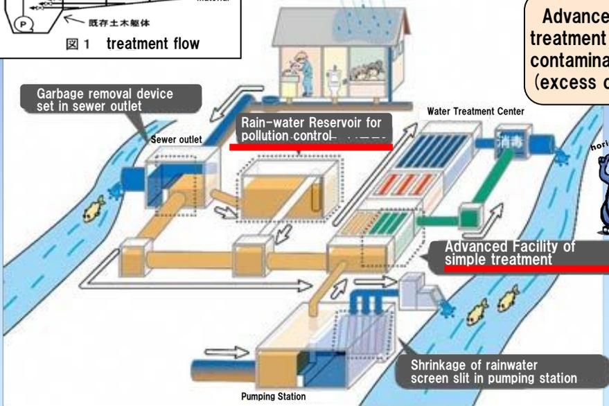
\*By replacing sedimentation tank to filtration facility, water quality improves substantially compared with conventional simple treatment.
