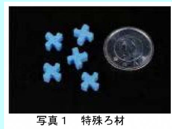
Pic.1 Special filter material
